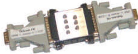
9-25 Adapter + MiniTester + 25-9 Adapter
