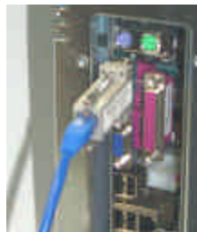
PC with DB9 to RJ45 Adapter and RJ45 Cable.
