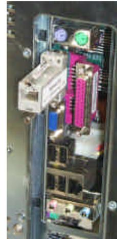
Once you have inserted the loopback plug, run the **Telcom FX Loopback Test Software**. See below for availability of software.
