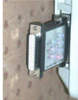
Mini-Tester inserted into SMDR Port
